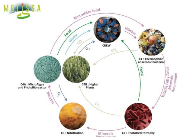
Figure 7. A schematic representation of the MELiSSA loop (courtesy of the MELiSSA Foundation)
