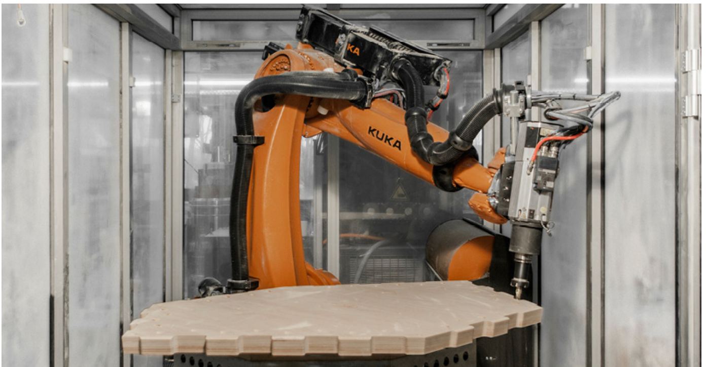
Figure 39: Kuka robot cutting a plywood panel for the Landesgartenschau Exhibition Hall
