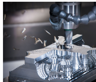
Figure 31: Aluminum Slab Milling
