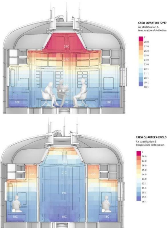
Fig. 17. Level 2 - Air Stratification & Temperature Analysis
