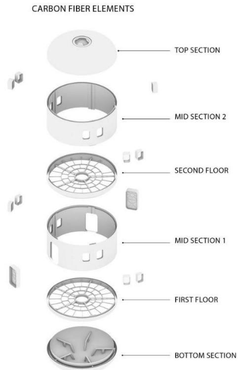
Fig. 6. Carbon Fiber Structural Elements
