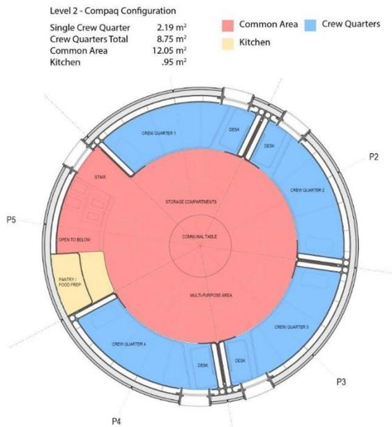
Fig. 10. Level 2 Floor Plan
